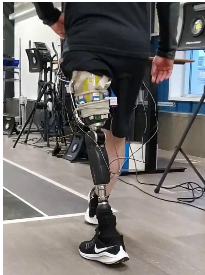
Figure 2 Amputee walking with SocketSense system integrated with their prosthesis.
