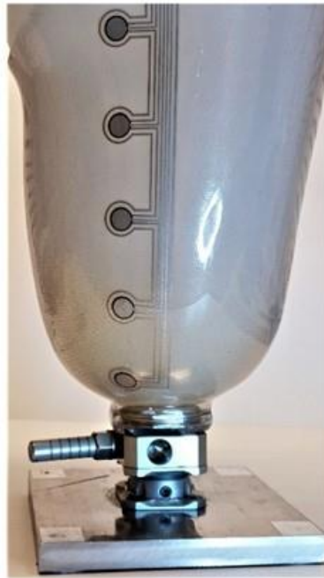
Figure 7 Liner inflated inside a prosthetic socket to apply specified uniform pressure on the sensors integrated in the socket
